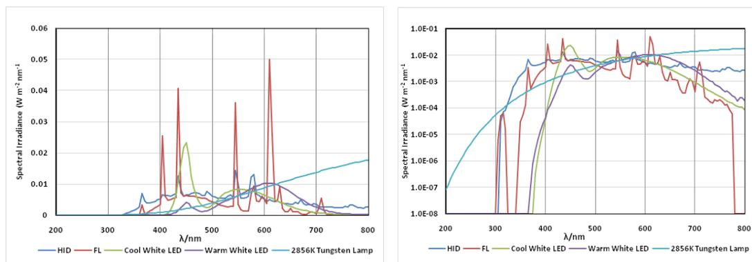
Figure 1. Spectral irradiance distributions of typical lighting sources
